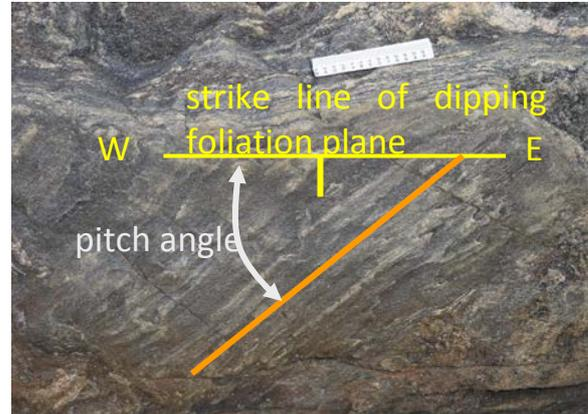
It may be more accurate to measure a line as a pitch, particularly if the line is to be later geometrically associated with the plane. Where the plane containing the line dips steeply then it is more accurate to measure the line as a pitch in the plane. It is generally best to measure fault slickenlines on slickensides this way as it ensures that the line orientation actually lies in the plane of the fault surface, which is required for some types of analysis.
