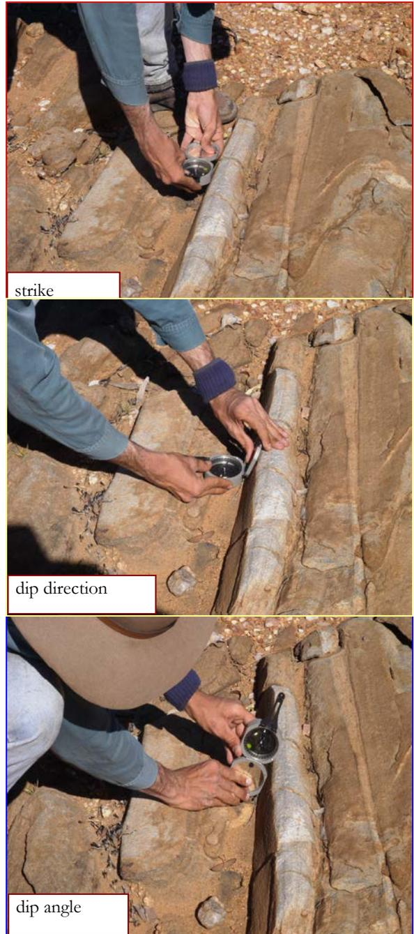
The example above shows measurement procedures using a Brunton compass. Although the principles remain the same, the procedure differs between compass types. The 'Clar'-type compass (also known as Breithaupt, or Frieberg compass), shown measuring dip and dip direction on the next page, uses a scale on the hinge so that only a single action is required to get both the dip direction and the dip angle. (Although the angle scale does not have the precision of the Brunton compass).
