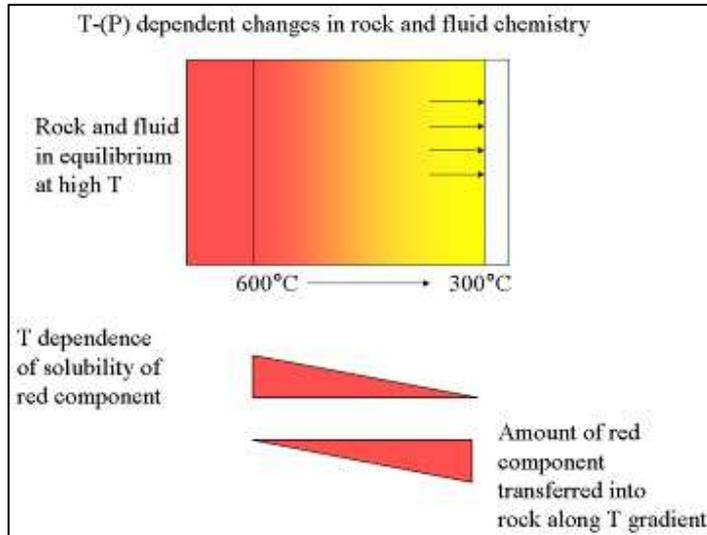
Figure 6: Schematic diagram showing the effect of allowing fluid to progressively equilibrate with a rock across a temperature (or pressure) gradient. E.g. down-temperature flow will cause silicification (yellow), up-temperature flow will cause silica dissolution. Such patterns can be recognised by regional sampling, and in some cases may correlate with the source-regions of major mineralized hydrothermal systems, although the links are very difficult to demonstrate.
